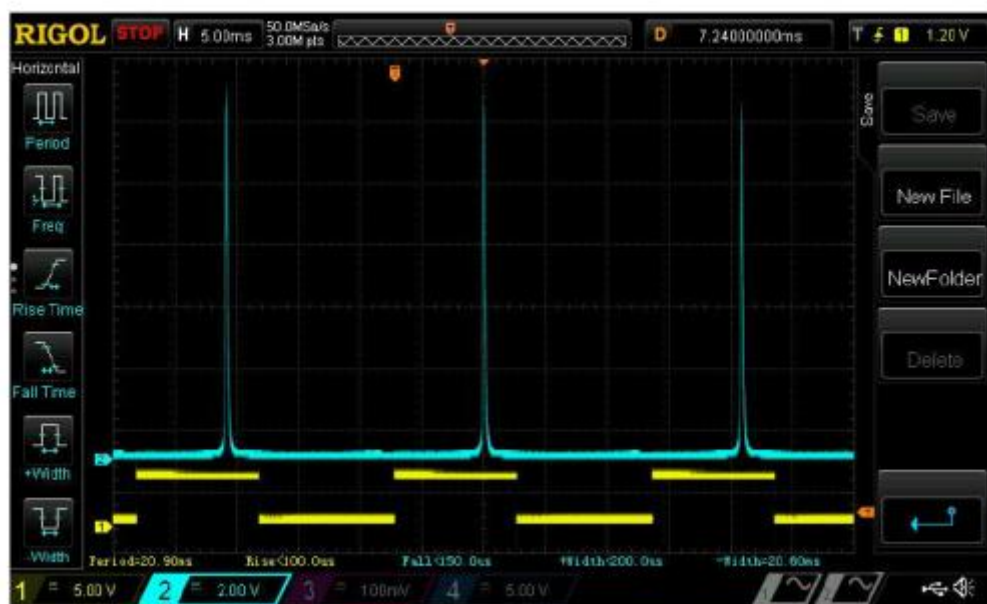
Linewidth measurement using Fabry-Perrot Interferometer
