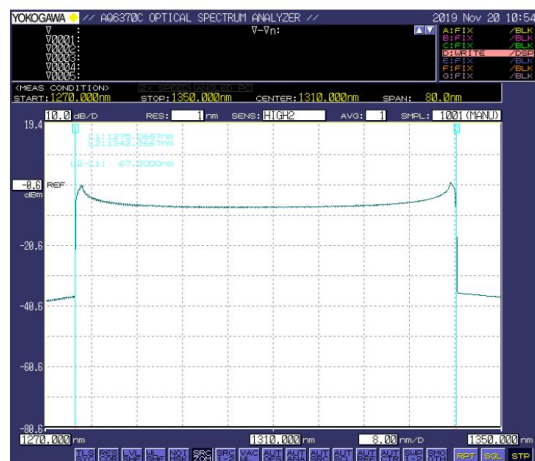
Swept laser spectrum at 1310nm.
