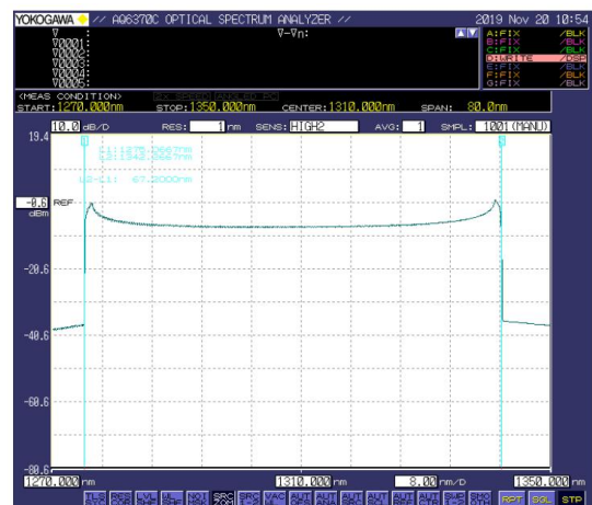
Swept laser spectrum at 1310nm.
