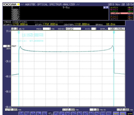
Swept laser spectrum at 1310nm.
