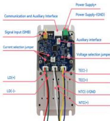
**Please be sure to refer to the laser manual, the wiring sequence of the corresponding connector, and the wiring on the circuit board to confirm that the laser is compatible with the current wiring sequence. Powering on with an incorrect wiring sequence may cause damage to the laser!**
