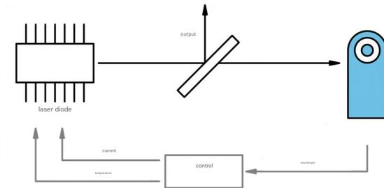
The compact wavelength meter can be used to stabilize the wavelength of tunable lasers, such as laser diodes. It provides an accurate and fast wavelength signal. Suitable control electronics can form a feedback loop to lock the wavelength and provide continuous tuning within the mode-hop-free tuning range of the laser diode.
