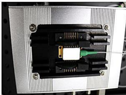
1550nm PM SLD Laser diode
