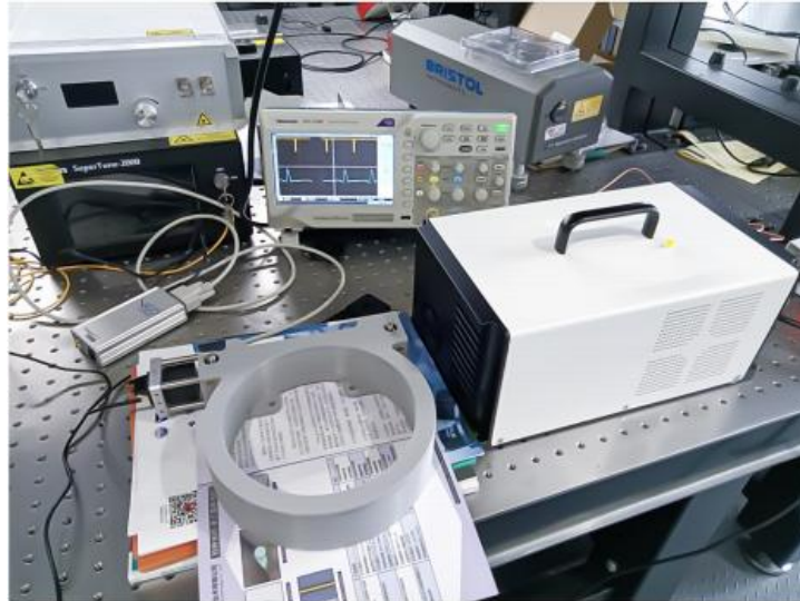
NF 3 gas absorption measurement experiment system diagram
